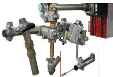
Seam tracking with sensing probe
