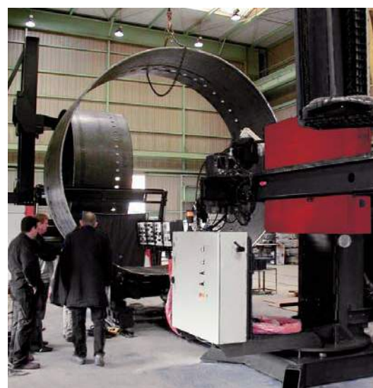
Large column and booms, rotators and positioners are proposed in this windmills solution.
