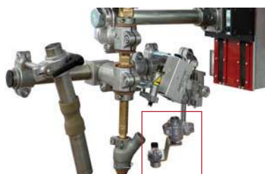
Seam tracking with inductive sensor
